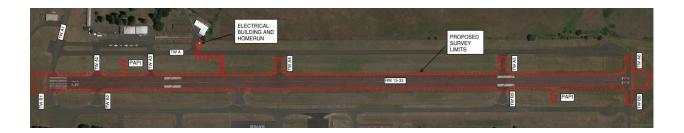
Survey data, on pavement, shall be collected at cross sections on a 25' (maximum) interval. interval. At each cross section, shots shall be taken on centerline, 12.5' from centerline, 25' from centerline, 37.5' from centerline, 50' from centerline, edge of pavement (on pavement), edge of pavement (on shoulder), then on a maximum 25' interval to approximately 50' from edge of pavement.
